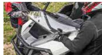
Offers fully-sealed or flipped-down venting options. Upper half detaches, leaving lower half for protection with maximum ventilation.
