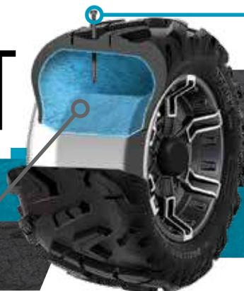
Once a leak occurs, the tyre sealant rushes out of the tyre and quickly creates a permanent solid plug.
