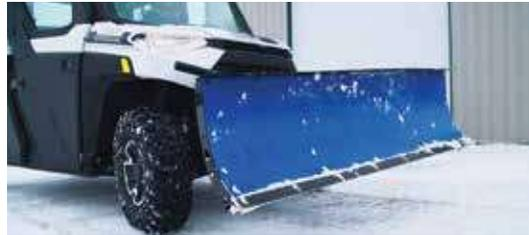
PLOW IS AUTOMATICALLY RAISED WHEN SHIFTING INTO REVERSE
